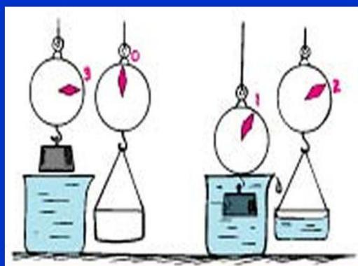
An immersed body is buoyed up by a force equal to the weight of the fluid it displaces
