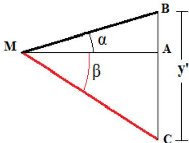
$$tg(\alpha) = \frac{AB}{MA} \Rightarrow AB = MA \times tg(\alpha) \dots\dots(1)$$
