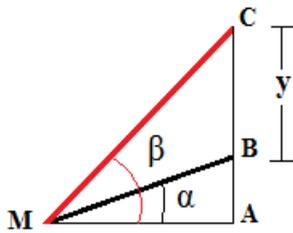
$$tg(\alpha) = \frac{AB}{MA} \Rightarrow AB = MA \times tg(\alpha) \dots\dots(1)$$
