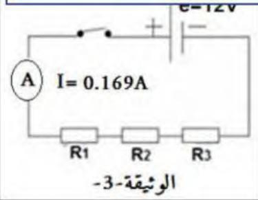
لدينا:  $R_t = R_1 + R_2 + R_3$  ,  $R_3 = R_t - (R_1 + R_2) = 71 - (27 + 15) = 29 \Omega$
