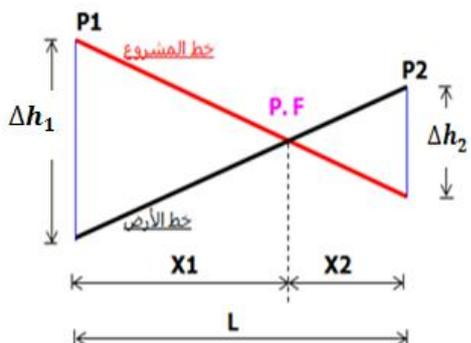
$$\frac{X_1}{\Delta h_1} = \frac{X_2}{\Delta h_2} = \frac{X_1 + X_2}{\Delta h_1 + \Delta h_2} = \frac{l}{\Delta h_T}$$
