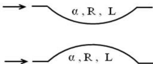
$$\begin{aligned} 2\pi R &\rightarrow 360^\circ \\ L &\rightarrow \alpha^\circ \\ \Rightarrow L &= \frac{\pi \cdot R \cdot \alpha^\circ}{180^\circ} \end{aligned}$$
