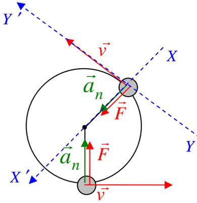
$$F = m \frac{v^2}{r} \quad \dots\dots\dots(1)' \quad \Leftarrow F = m \cdot a_n$$
