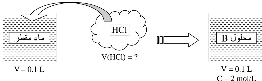
$$\begin{aligned} C &= \frac{n(\text{HCl})}{V} = \frac{\frac{V_{(\text{HCl})}}{M}}{V} = \frac{V_{(\text{HCl})}}{M \cdot V} \rightarrow V_{(\text{HCl})} = C \cdot M \cdot V \\ V_{(\text{HCl})} &= 2 \cdot 22.4 \cdot 0.1 = 4.48 \text{ L} \end{aligned}$$
