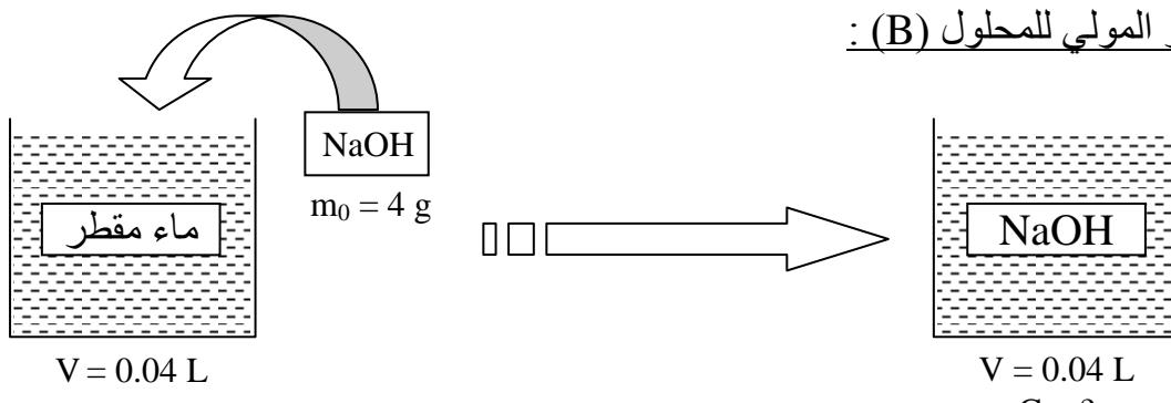
$$C = \frac{n_0(\text{NaOH})}{V} = \frac{\frac{m_0(\text{NaOH})}{M}}{V} = \frac{m_0(\text{NaOH})}{M.V}$$
